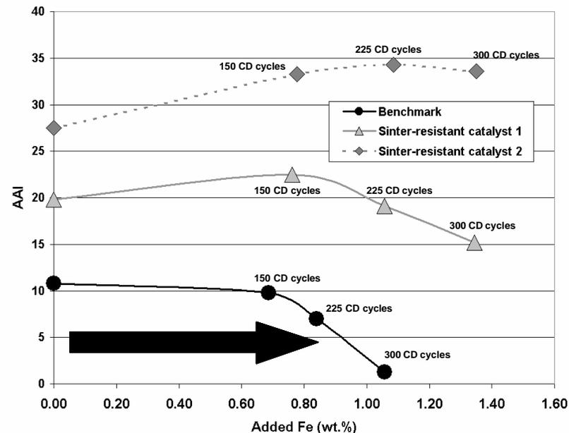
**Figure 1.** Absolute AAI as a function of Fe addition during the CD-ALFA deactivation process for three catalysts.
