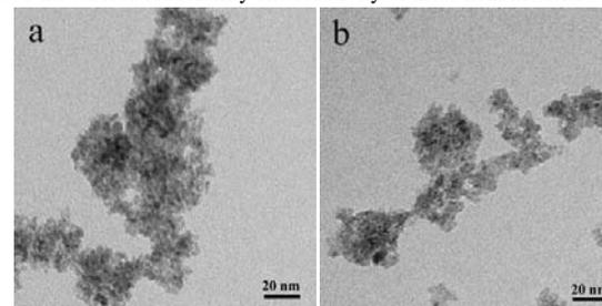
**Figure 1.** TEM images of 2.6 nm CeO<sub>2</sub> nanoparticles via thermolysis method (a) and 3.0 nm CeO<sub>2</sub> nanoparticles via hydrolysis method (b).
